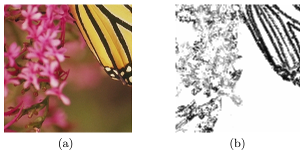
Figure 1. Re-representation in computer vision. Raw pixel data in (a) is re-represented in (b) in a form that facilitates image analysis and understanding via computer vision algorithms, encoding such information as edge location, or, as in this case, a local point spread function.
