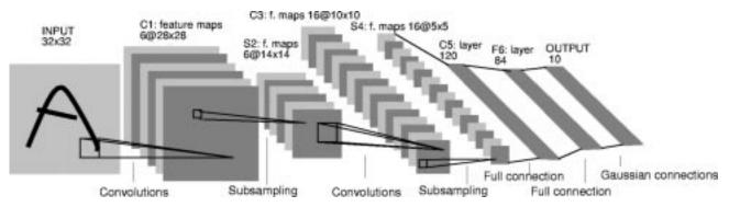
**Fig. 2.** Architecture of LeNet-5, a convolutional NN, here used for digits recognition. Each plane is a feature map, i.e., a set of units whose weights are constrained to be identical.
