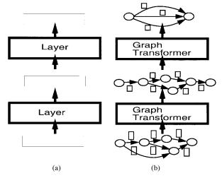
**Fig. 15.** Traditional NN's and multimodule systems communicate fixed-size vectors between layers. Multilayer GTN's are composed of trainable modules that operate on and produce graphs whose arcs carry numerical information.
