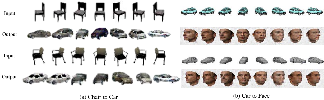
Figure 8. Discovering relations of images from visually very different object classes. (a) chair to car translation. DiscoGAN is trained on chair and car images (b) car to face translation. DiscoGAN is trained on car and face images. Our model successfully pairs images with similar orientation.
